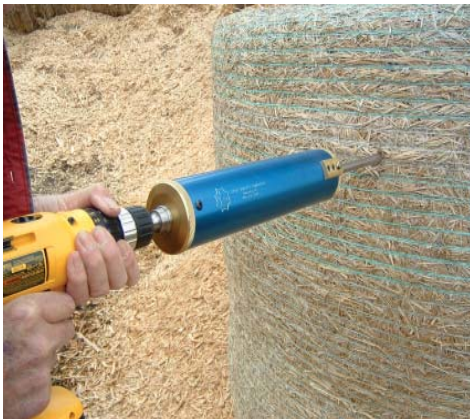
Taking a core sample with drill (14 volt or greater is recommended)
